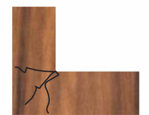
Cutting a laminate sheet at an angle of 90° degree leads to development of cracks in corner after pasting. Therefore it is advisable to avoid cutting at an angle of 90° degrees.
